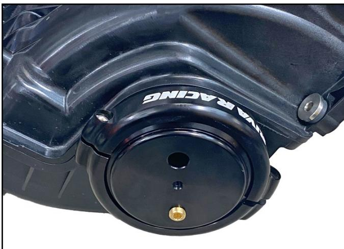
Place one half of the block-off clamp with RIVA logo on top of the block-off insert. Place other half of block-off clamp with 3 cut outs onto bottom of block-off insert so the cut outs are against the intake manifold.
