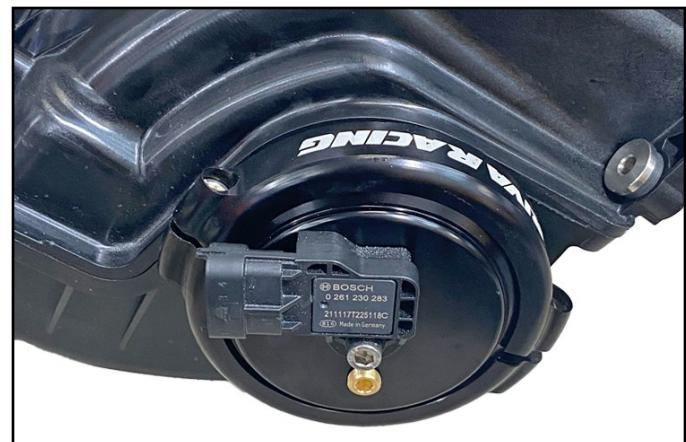
Install MAPTS sensor and secure using supplied M6 bolt and washer. **NOTE: Verify o-ring is in place on sensor.**
