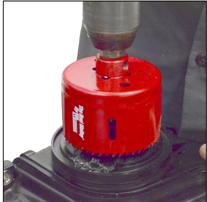
Hold manifold securely and drill slowly. **NOTE: Take your time! Do not force.** Internal filter element is directly behind the thin section you are drilling into.
